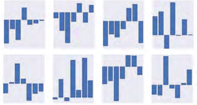
Figure 3: Convolution weights learned by the CNN on the step count time series of the UPTAKE dataset. Each graph shows the 7 learned weights for each of the nodes in the first convolutional layer for step counts.
